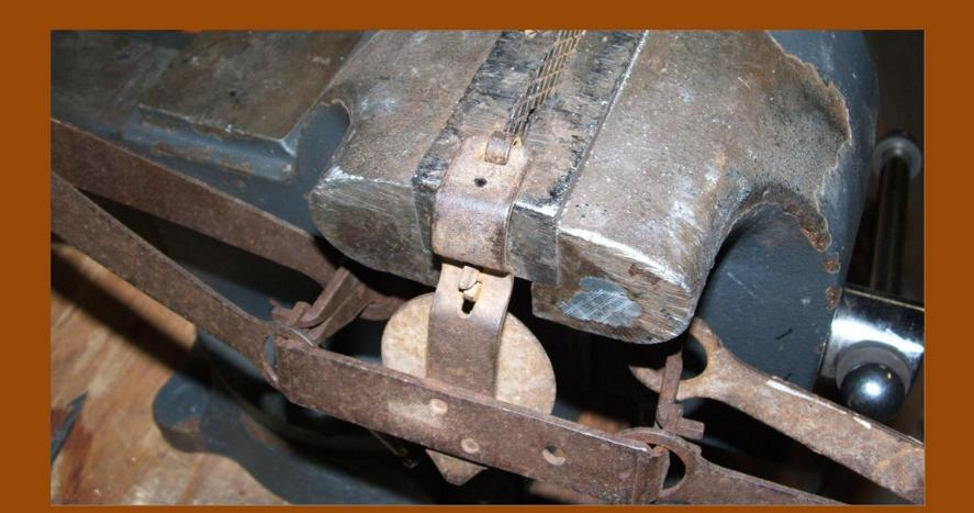
It's best to start with a pilot hole, I started with an 1/8" bit first. Size the bit just a little bigger than the size of the J-hook , this hook was 7/32", so I used a 15/64" bit, just under ¼". You could probably get away with ¼", but check it first , you just want enough movement to swivel.
