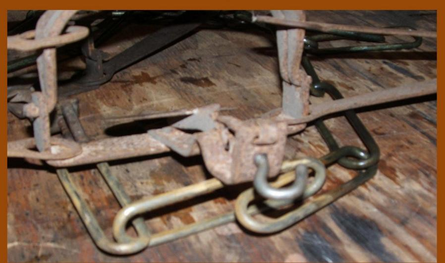
Here are some of the modern J-hooks and modern swivels that can be bought through trap suppliers. These hooks are made of a good steel. These are not often bought to replace broken ones, they are most commonly used to add a swivel section into a chain. Rarely would one of these bend or break.
