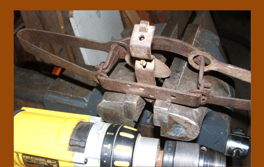
After it's drilled and the hook is slipped in , set the trap just to make sure nothing gets in the way of the dog and trigger. If it's centered up right, even on this #2 there is good room for the J-hook.
