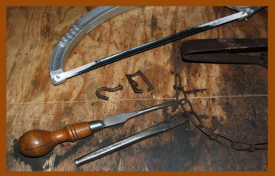
It's much easier if you have a vise, if not this is going to get clumsy. Mark the location to drill a hole under the dog slot, be careful to get this centered up so it doesn't interfere with the movement of the dog. Don't get too low or the swivel will hang up in the bend of the bar.
